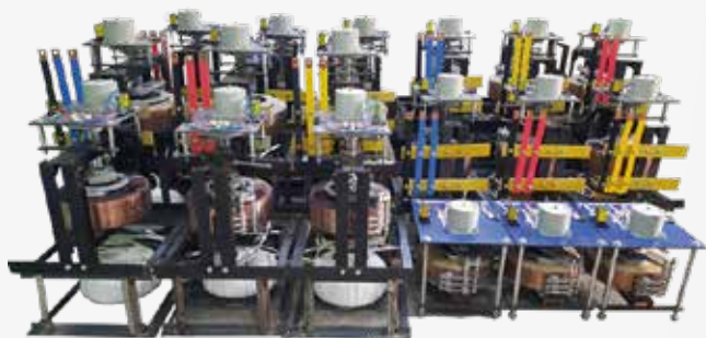
INTERNAL SECTION OF SERVO CONTROL VOLTAGE STABILIZER
