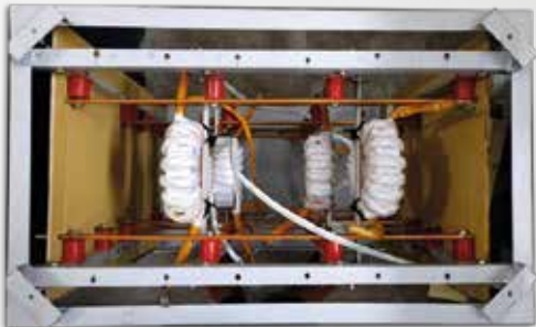
INTERNAL SECTION OF SERVO CONTROL VOLTAGE STABILIZER
